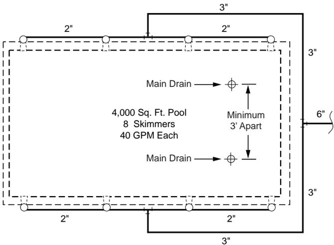
**Acceptable Flow Rate (10-60 GPM)**
