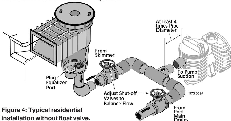
**Figure 4: Typical residential installation without float valve. Use with at least two main drains.**
